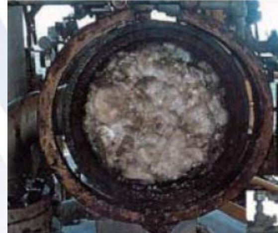
A large gas hydrate plug formed in a sub sea hydrocarbon pipeline (Petrobras, Brazil)(Naval Research Laboratory)
