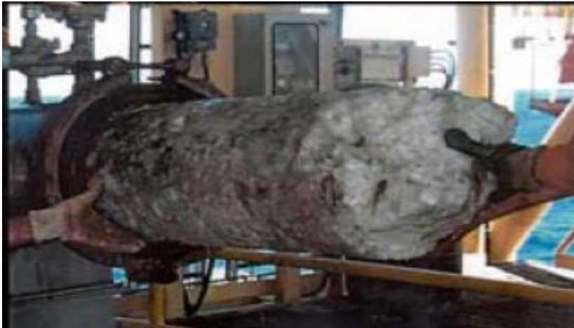
A large gas hydrate plug formed in a sub sea hydrocarbon pipeline (Petrobras, Brazil)(Naval Research Laboratory)
